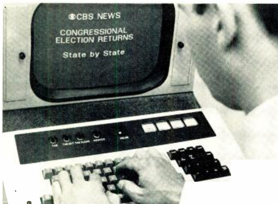
CBS Labs Vidifont char. generator produces many type fonts, sizes, logos in real time.
