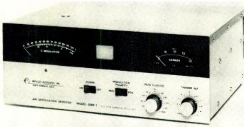
Moseley remote AM modulation monitor AMR-1 uses FETs, has 10-kHz notch filter.
